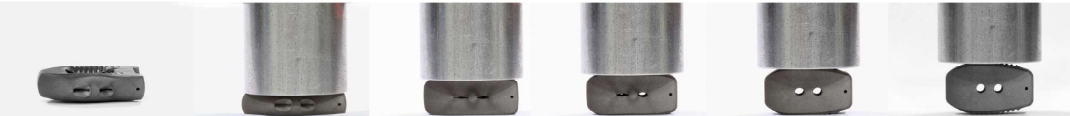
Internal testing: plastic deformation of implant fails to dislodge FGOIC Ti - no flaking and no sharp debris
