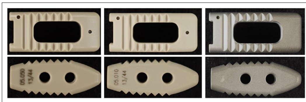
Figure 1. Uncoated PLIF PEEK cage (left), CaP nanocoated PLIF PEEK cage (middle; the coating is not visible to the naked eye), titanium nanocoated PLIF PEEK cage (right) used for testing.
